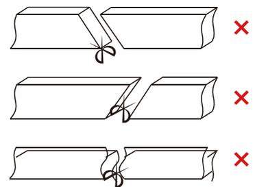
Please do not arbitrarily cut or cut into a bevel and arc section.
