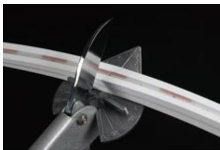
Make precise vertical cuts at the exact cut position of the light strip.
