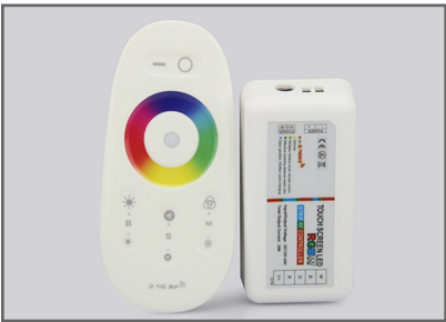
RGB+W controller: 4 Channel DC12V/24V, 6A, RGB+W, RF remote with finger touch ring.
