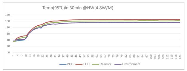
The above curves indicate the temp. changing in LED,resistor & PCB within 120 minutes after powering on, under the ambient temperature of 95°C.
