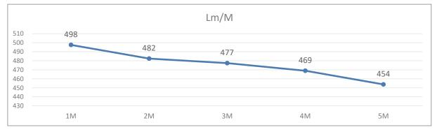
From above chart, please connect 5M at most by one-end power to keep brightness consistency.
