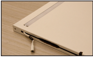
Embed the finished lamp into the board, and reserve a groove for the wire on the side.
