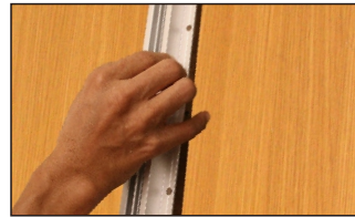
Fix STR002 to the groove.
