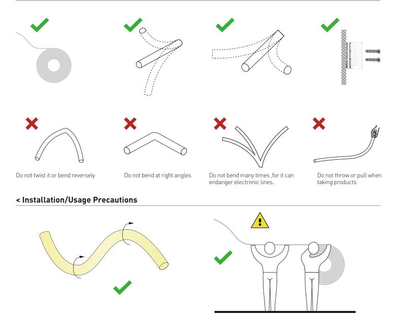
Bending diameter should be more than  $\phi$ 100mm
