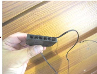
Step III: Put the RU plug into splitter box.
