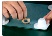
2: Fix the sensor with 3M tape on the back of the mirror.
