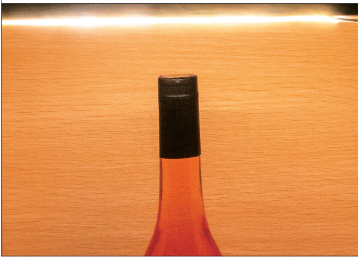
New COB Strip without any LED dots
