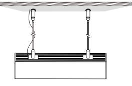
Fix the top joiner to the ceiling. Adjust the cable length to suit
